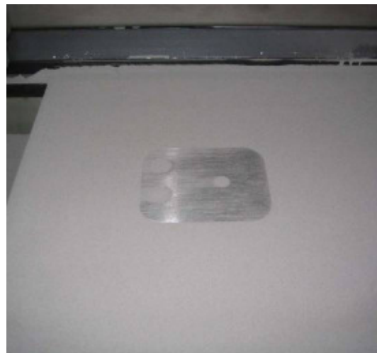
5. Top surface of preform positioned at building plane ( Z=0 ) in powder bed
