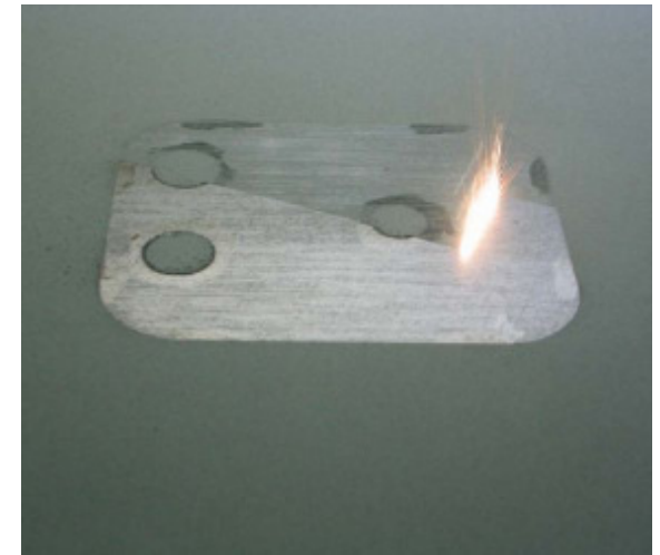
6. Building starts with first layer exposed onto top of preform, creating a metallurgical bonding
