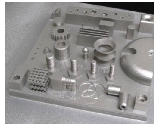
Benchmark test geometry in EOS StainlessSteel 17-4. Source: NASA / General Pattern.
