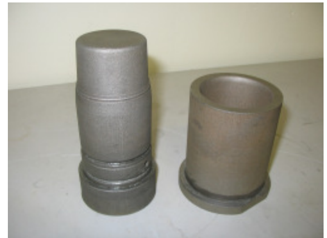
DirectTool piston and cavity built on EOSINT M system. Diameter 60mm, height 130mm.
