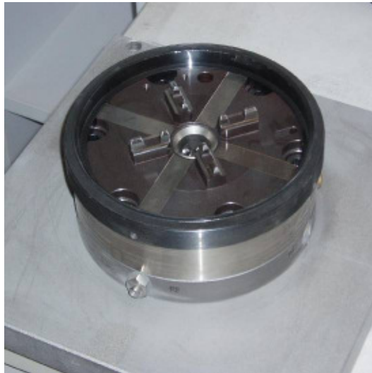
1. Erowa Powerchuck 150 unit fits onto platform carrier in M270 process chamber
