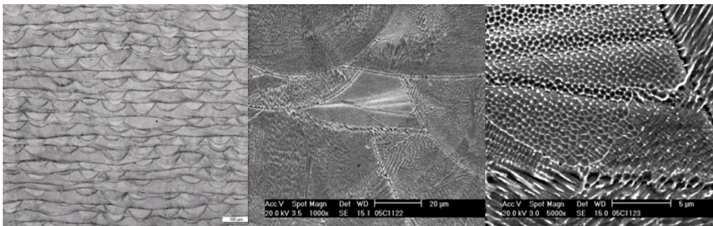
Fig 2: CobaltChrome MP1 samples, laser-sintered on EOSINT M 270 and etched. (a) 10x optical micrograph. (b) 1000x SEM micrograph. (c) 5000x SEM.
