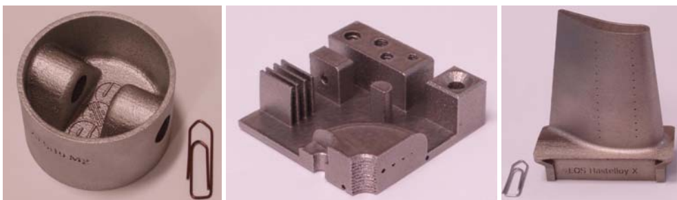
Fig. 4. Parts built on EOSINT M 270 systems: (a) AISi10Mg, (b) Inconel 718, (c) Hastalloy X.
