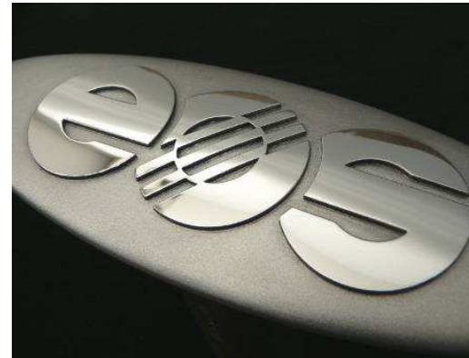
Demonstration part in EOS StainlessSteel GP1, partly polished
