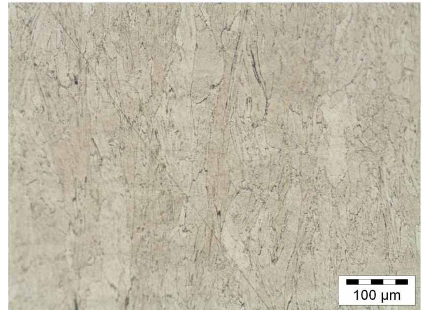
Vertical cross-sections through EOS NickelAlloy IN718 parts, etched.
