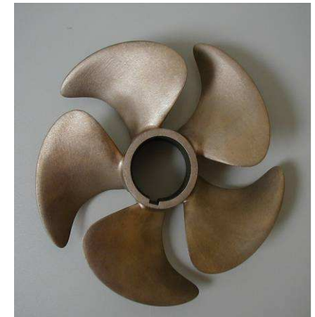
propeller prototype for wind tunnel testing
