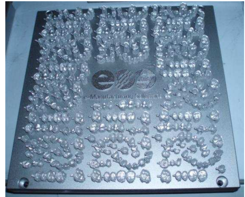
Job in EOS CobaltChrome SP2 with 384 units of dental restorations. Building time 20h.
