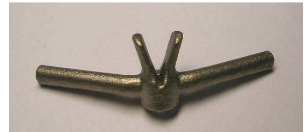
Spinal implant built in EOS Titanium Ti64
